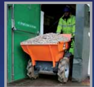
Designed To Fit Through Standard Doorways
