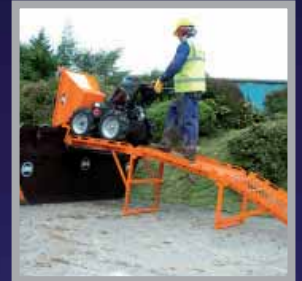
Enables Tipping Directly Into Skip
