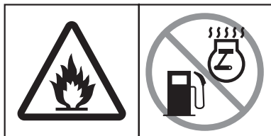
Petrol is highly flammable. Turn off the engine and allow time to cool before refuelling.
